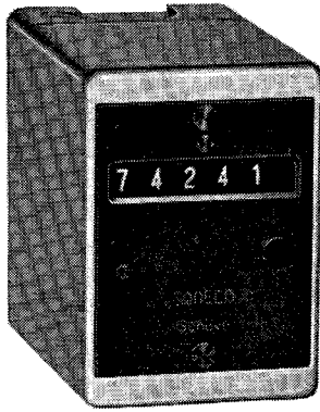
TCeB... Small Impulse Counters with very reduced case depth 4, 5, 6 or 7 digits – flush panel or projection mounting – with or without manual zero reset – 10 or 25 imp/sec
