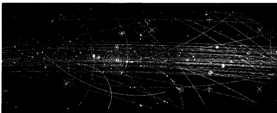
A bubble chamber photograph, taken on the CERN 2 metre hydrogen chamber, which gives some indication of the problems of extracting information of particle behaviour from these experiments. The photographs must be 'scanned' to identify interesting events, these events must then be accurately measured, and these measurements, in combination with thousands of others, must be analysed by the computer.
